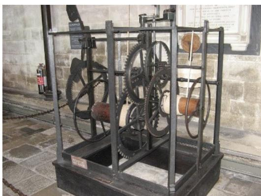
The cathedral's website claims that it is "probably the oldest working mechanical clock in existence, made of hand-wrought iron in, or before, 1386."
